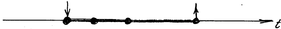
Figure 3.2.5.2. Time diagram illustrating a typical case of symbol manipulation. The symbolic processor is idle until a symbol arrives into the input zone. This triggers a sequence of three symbolic operations that result in the production and emission of another symbol.
